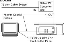
The cable hook-up shown at the bottom left allows VCR-TV functions except for viewing one channel while recording another.
